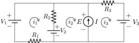
A13: List the unknowns in the linear system for this circuit using the technique of loop currents you learned in the lectures and computer labs this term.
